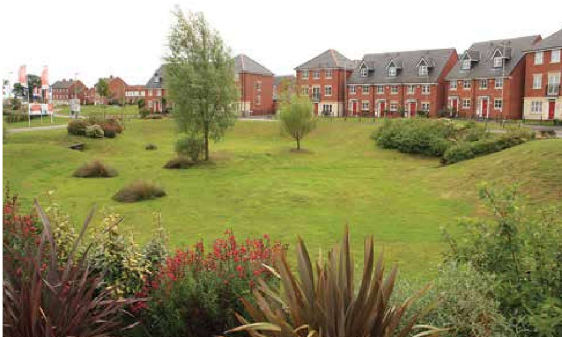
Figure 4-5: Detention Basin Example (ref. SUDS Manual)
