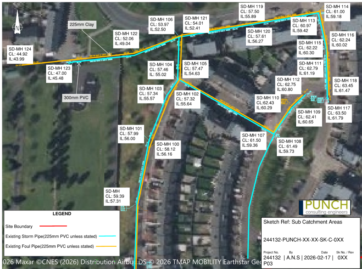
Figure 2-3 Existing Storm & Foul Drainage in Glentrasna, to the north (extract from survey)
