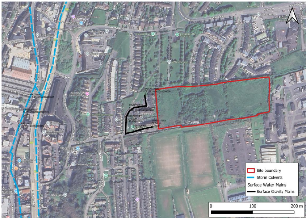
Figure 2-1: Existing storm drainage adjacent to site (extract from UE records, site boundary outlined in red)
