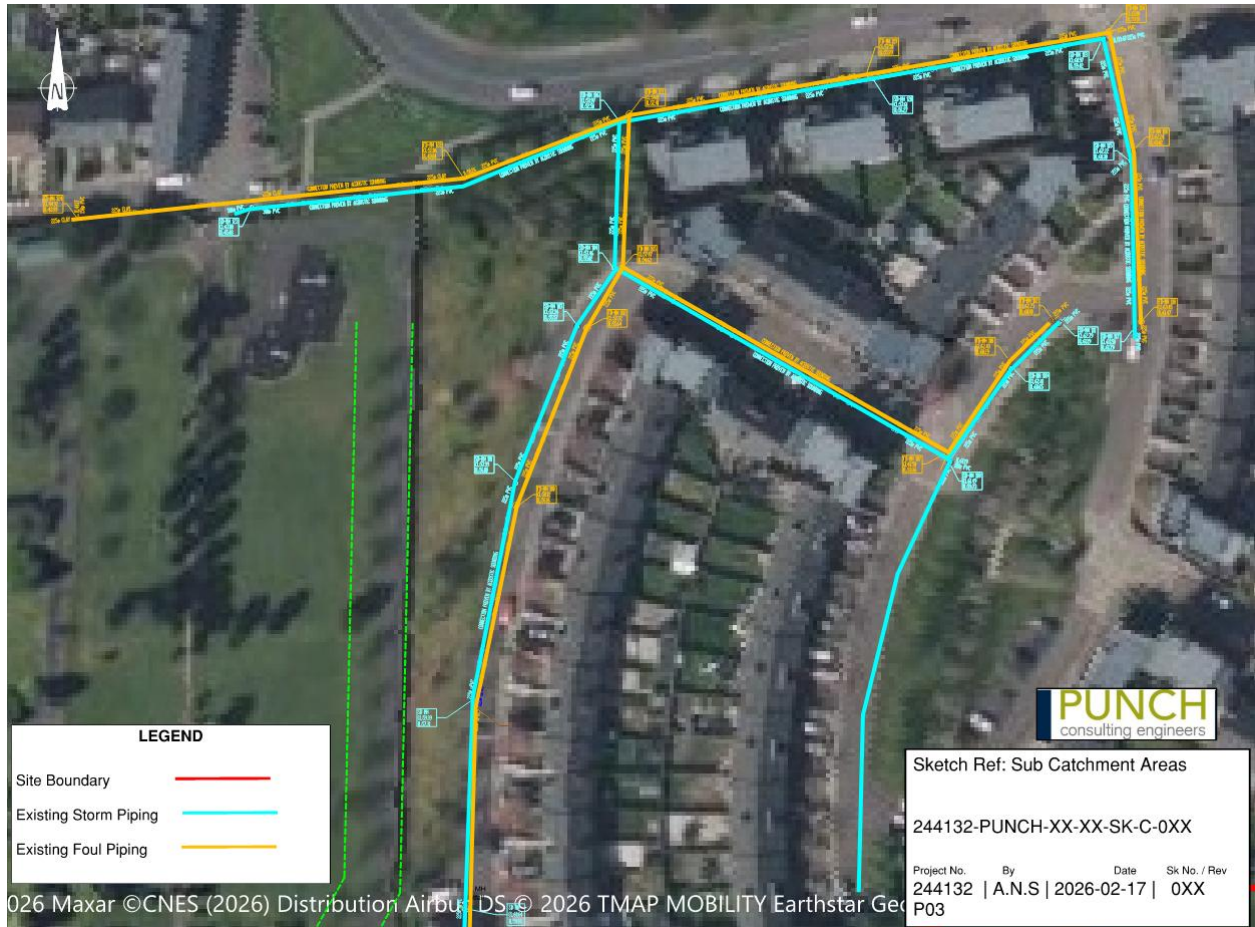
Figure 3-7 Existing Storm Drainage in Glentrasna Estate, to the north (extract from GPR survey)
